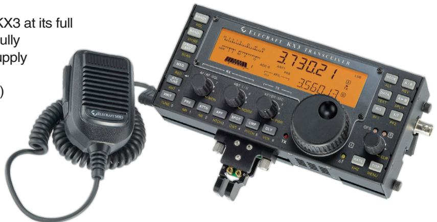
decreases as the voltage increases. For 5 W operation, the KX3 supply voltage can range from 9 to 15 V dc, and power supply current is significantly lower at 15 V than at 9 V. This is probably because efficient switching voltage regulators are used for some of the radio circuitry. Switchers draw approximately the same power independent of the input voltage, so current goes down as voltage goes up.
